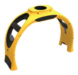
The single-piece Frame attaches to the Backboard and holds the Compression Module in position over the patient. With the Backboard attached, the Frame is designed to create a rigid structure that enables a consistent compression depth without unwanted flex or distortion during operation. The latches are self-centering and self-locking and are easy to match up with, and snap into, the Backboard.
