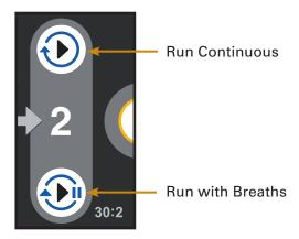
To temporarily stop compressions for any reason, press the pause button. If necessary, make adjustments to the Piston position using the Adjust Up/Down Buttons so that it is making firm contact with the patient's chest. To resume compressions, push the "Run Continuous" button OR the "Run with Breaths" button.
