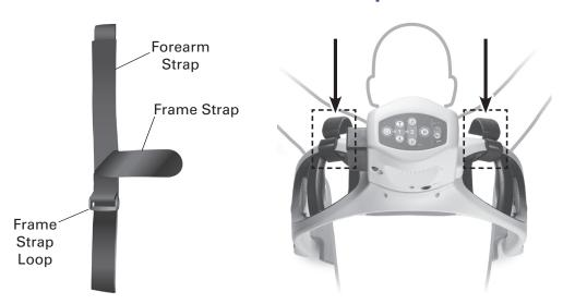
The Patient Wrist Straps attach a patient's arms to the Lifeline ARM device for ease of transporting the patient and the unit together. As shown in the above left illustration, each Patient Wrist Strap is comprised of two main strap sections: a Frame Strap that attaches to the Frame and a Forearm Strap that wraps around the patient's wrist.
